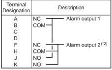
When output is not used, the terminals are opened. \*2: Except SKYD-1 type.
